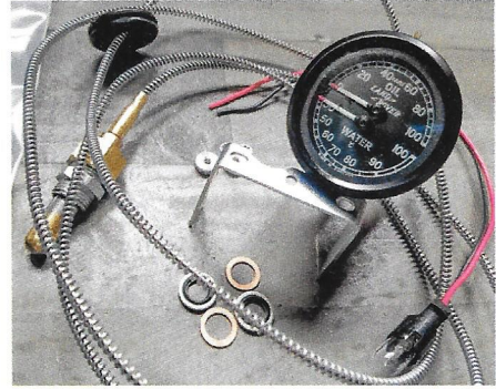
3. Gauge kit gauge comes with a permanently attached capillary tube and a choice of two threaded adapters (3/8NPT or 5/8UNF) to fit most engine blocks
