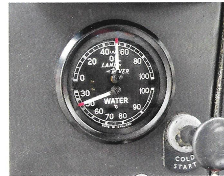
12. Installed mechanical Smiths gauge shows accurate oil pressure and water temperature on engine start-up
