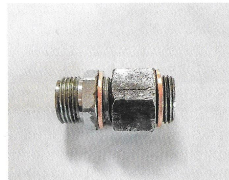
9. The water temperature bulb required an adapter from 5/8UNF (L) to the 3/8BSP thread (R) in my engine block. I used copper washers between all connections
